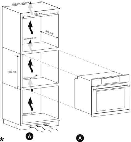
**EN** If the furniture is coverage with a bottom at the back part, provide an opening for the power supply cable.
