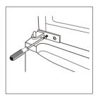
10. Place the upper door back on. Ensure the door is aligned horizontally and vertically so that the seal are closed on all sides before finally tightening the top hinge. Then inert the top hinge and screw it to the top of unit and then fix hinge cover (in accessary bag) by screw.
