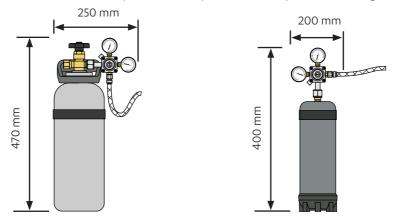
Secure cylinder vertically to a robust surface with the hook & loop strap and bracket supplied.
