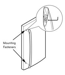
2 Place the handle on the door by aligning handle footprints to fit mounting fasteners and tighten the set screws on the bottom of the handle with a 3.1 mm (1/8") Allen wrench.
