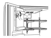
To remove the in-door ice bin, grip the front handle, slightly lift the lower part, and slowly pull out the bin as shown.
