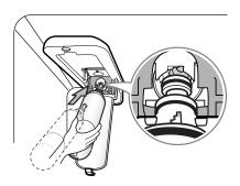
· Rotate the water filter up into position and close the cover. The cover will click when closed correctly.
