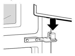
1 Lower the door onto the middle hinge pin. Make sure that the plastic sleeve is inserted into the bottom of the door.
