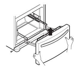
5 With both hands, flex the center bar enough to allow the gears on both ends to release from the track.
