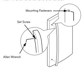
2 Loosen the set screws located on the lower side of the handle with a 3.1 mm (1/8") Allen wrench and remove the handle.
