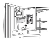
2 Avoid touching the ice-detecting sensor when replacing the ice bin. See the label on the ice compartment door for details.
