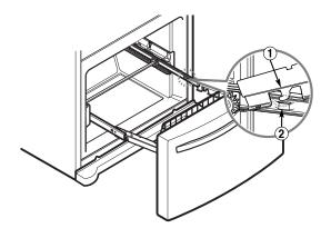
3 Lower door into final position and tighten the screws ③. Make sure you have a right rail cover for each side.
