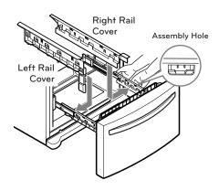
5 With the drawer pulled out to full extension, insert the lower basket in the rail assembly.
