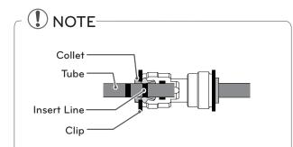
1) Gently press the Collet and insert the tube until only one line shows on the tube.
