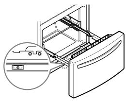
4 With both hands, hold both sides of the door and pull it up to separate it from the rails.
