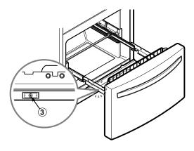
4 Align the top holes of the rail cover with the top holes of the door supports to assemble the rail covers.
