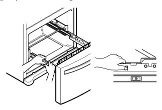
3 Remove the screws of the rail on both sides.
