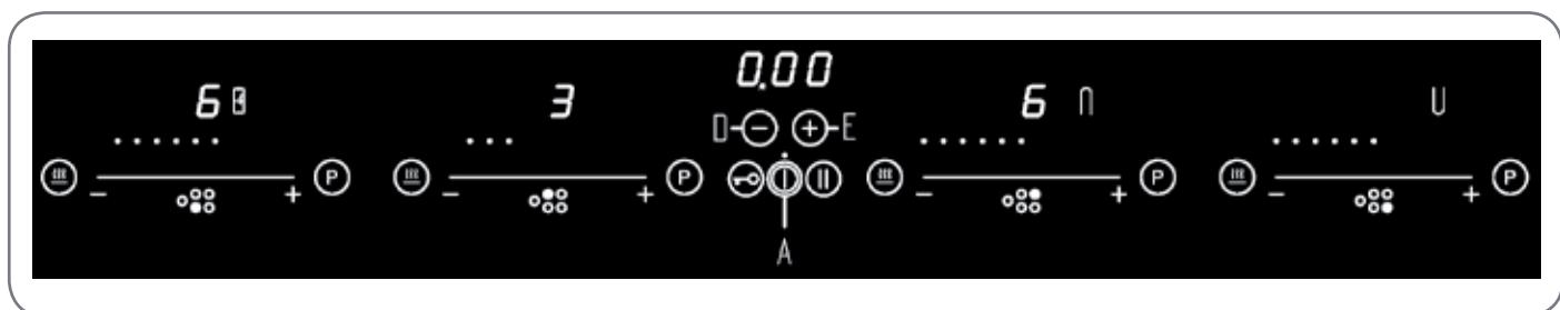
Simultaneously press (D + E) as many times as necessary to select the alarm. The respective LED is located between the keys (E) and (D).
