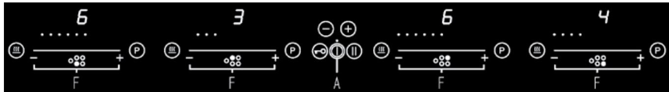
If a specific point of slide control is pressed for at least 3 seconds, the automatic cooking is activated (see Automatic fast heating).
