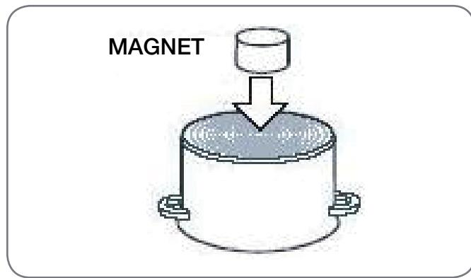
Use small magnet to test if the dish bottom is magnetic. Only dishes where magnet sticks to the bottom are suitable for induction cooking.
