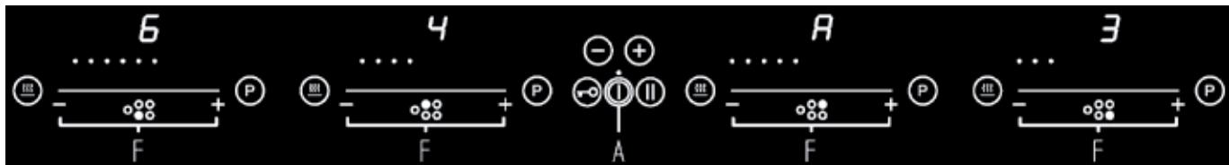
Once the time from the chart below expires, the function is switched off and "A" disappears. You can also switch the automatic cooking mode off anytime by bringing power setting to "0".
