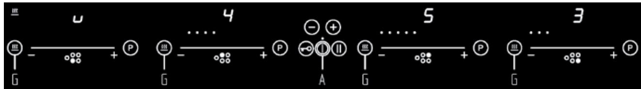
If the special function key is pressed a fourth time the warming function ends.
