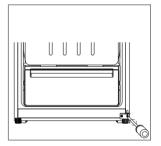
8.Disassemble right hinge, find out right bottom hinge from spare parts bags and fix it.
