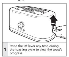
**TIP:** For smaller items, lift up on the lift lever to raise toast above the top of the Toaster.
