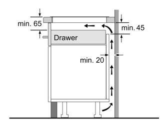
\_ min. 550 Measurements in mm
