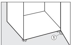
■ Ensure that you unscrew the adjustable foot ① from the lower hinge plate with the enclosed spanner until it sits on the floor. Then unscrew the foot by a further ¼ turn.
