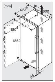
x: Dimensions without wall spacers fitted. Appliance depth is increased by 35 mm with the wall spacers supplied fitted.
