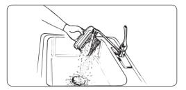
Rinse the dirty water tank and filter thoroughly with warm water. You should allow them to dry fully before replacing them on your cleaner to prevent mildew.
