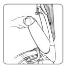
Tilt the solution reservoir away from the cleaner and remove.
