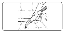
Turn power switch on and brush bar switch off. While depressing the solution spray trigger, pull attachment in backward motion. Release trigger and push attachment forward over the same path to remove dirty water and solution from upholstery. (For heavily soiled areas, repeat if necessary).
