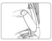
Place the bottom of the solution reservoir into the cleaner and push into place. There will be an audible click when the reservoir is in the correct position.
