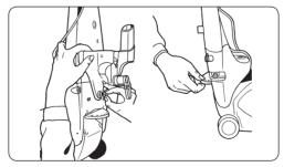
Place nut into recess on tool caddy and hold into Place screw through place. Press handle release with your other hand centre of lower to tilt the mid section backwards.
