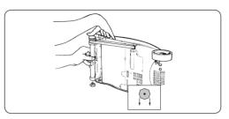
When replacing the belt, first slide it onto the motor shaft. Then slip the brush roll through the belt. Place the belt in the area of the brush without bristles. Slide the brush roll into the nozzle, ensuring that the brush roll end caps are orientated correctly, see inset picture. Manually turn the brush roll to check that it is fitted properly.
