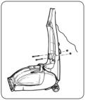
Insert the two nuts into the recesses located on the left and right holding the nuts in place, insert the two medium length screws through the front of the mid section and tiahten.
