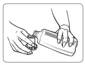
Fill the measuring cap 3 times with VAX AAA carpet cleaning solution and pour into the reservoir. Note: The cleaning solution supplied with your machine is VAX AAA Carpet Cleaner. When replenishing this item, please use VAX Carpet Cleaner, which is available in 1 litre bottles from your VAX stockist.
