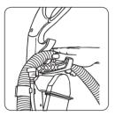
Run the hose to the upper caddy and press into hose clip #1. (See image above for hose clip position.)
