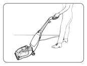
While pressing the solution release trigger, pull the cleaner in a backward motion. Release the trigger and push forward over the same path to remove the dirty water and solution from the carpet. Repeat if necessary. For best results use a smooth steady action - keeping the nozzle flat against the carpet. When the dirty water reaches the max fill line on the dirty water tank, empty the tank.
