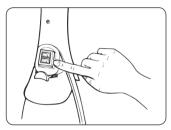
Plug the cord into a mains electricity socket. Turn the power and brush bar switches on. The switches are located on the front of the cleaner, above the solution reservoir. The power switch controls the vacuum motor and pump. The brush switch only turns the rotating brush bar on and off when the power switch is on.
