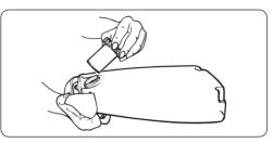
Unscrew the filler/measuring cap from the rear of the solution reservoir. Note: Always use the filler/measuring cap from the reservoir to determine precise solution quantity.
