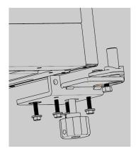
h) Get the lower left hinge from the accessory bag and install it on the bottom left hand side.
