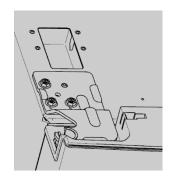
k) Get the upper left hinge from the accessory bag, fix it with bolts and install the ground wire(with a ring end) under one bolt. Connect red/yellow/blue cable socket from the
