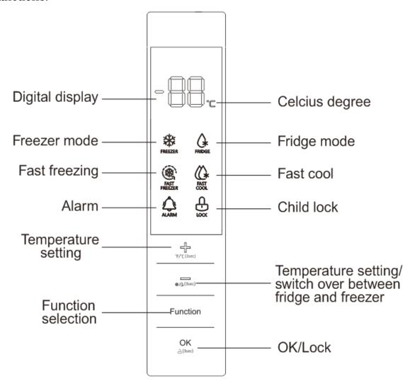
When the refrigerator is connected to power supply for the first time, all icons on the display panel gets illuminated for 2s, and the system runs in the freezer mode at - 18°C by default. When door is closed, the display will turn off automatically. It will light up if door is opened or any key is pressed.
