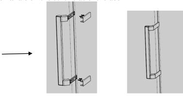
o) After the door handle is installed, the door reversing operation is finished.
