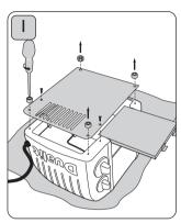
Unplug and place toaster on a soft cloth. Remove crumb tray and unscrew feet to remove the base plate.
