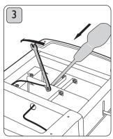
Unscrew brass links and wires.
