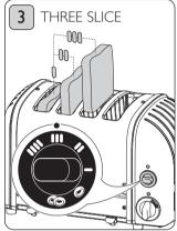
4 slot model: Rotate the 'selector switch' clockwise to the three slice indicator. The first three slots from the left will toast on both sides.
