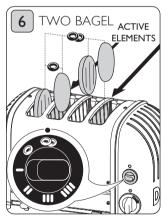
4 slot model: Rotate the 'selector switch' anti-clock-wise to the two bagel symbol. Only the second and forth element from the left will heat up.
