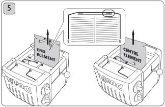
Remove element. To reassemble, reverse procedure ensuring wires and parts are correctly positioned. Ensure new element is marked the same as the one removed. The element heats on both sides and can be inserted facing either way. Check it is seated correctly in the channels either side. Portable Appliance Tested before use.
