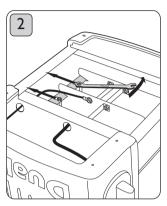
Loosen locking nuts on Unscr retaining plate using a 6.5mm wires. spanner and slide back. Ensure that the retaining plate is correctly in position when
