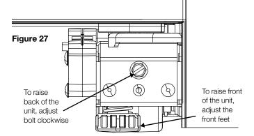
f. Adjust the leg levellers (Fig. 28) so that they touch the ground and can't be rotated further by bare hands. This will stop the refrigerator rolling forward when opening the doors.
