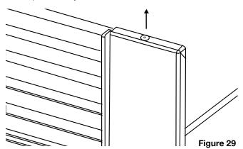
h. Drill dia 3.2mm pilot holes on the cabinetry and secure the Top Trim to the cabinetry using two screws each on left and right ends.
