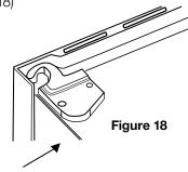
b. Remove the two screws shown. Attach the bracket to the top hinge using the removed screws.Recommended screw torque 8Nm.
