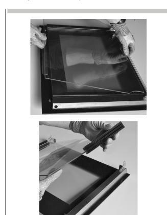
Replace the middle panes after cleaning in reverse order, checking that they are oriented so the words INTERNAL SIDE are properly legible.
