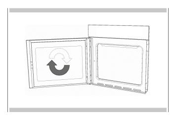
6. Secure the door in its new position using the 4 screws removed previously.
