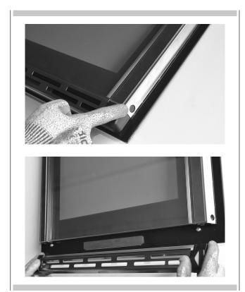
4. Slide out the internal glass as shown below. Remove the second and third panes of glass (middle panes) for cleaning sliding out the rubber strip.
