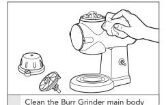
and all its parts by hand only. Wash with a soft, damp cloth. Dry thoroughly with a soft dry cloth. Do not wash in the dishwasher. Do not immerse in water.
