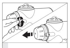
Remove the faceplate assembly by 3 loosening the screws on either side. Screws can be loosened by hand.
