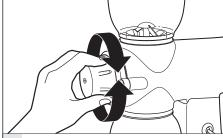
For maximum grind fineness: Turn the grind control dial to level 8.
