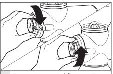
For maximum grind fineness: Turn the grind control gear clockwise, one "click" at a time until you hear a distinct grating or rubbing sound that signifies the burrs are touching. Then, turn the grind control gear one "click" counterclockwise. The grating or rubbing sound will stop.
