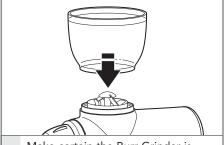
Make certain the Burr Grinder is unplugged. Attach the bean hopper to the top of the motor housing, turning clockwise until snug.
