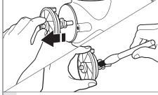
Pull the burr-shaft assembly out to clean with the other parts. Using the burr-cleaning brush, clean the burr mounted on the burr-shaft assembly and the burr mounted in the motor housing.
