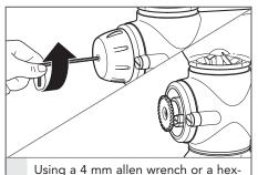
head screwdriver, remove the screw from the front of the grind control **3** dial by turning it counterclockwise. You will be able to see the grind control gear after the dial is removed.
