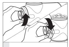
For maximum grind coarseness: Turn the grind control gear 5b counterclockwise, one "click" at a time until the clicking sound diminishes and the gear offers little resistance to being turned.
