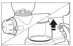
Make sure the bean hopper is empty; then, flip the POWER switch 1 up to turn on and run for a few seconds to clear any debris.
