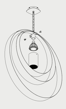
4. Unscrew the bolt off the inner ring, bring the inner ring to the Lunar Large body and screw into place securely.
