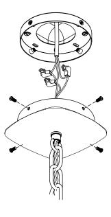
Unscrew the two thumb-turn screws from the top of the can and gently lower down the can.
