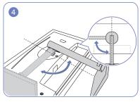
Turn the stand neck of the display clockwise for 90° to ensure that the stand neck of the display is put into place.
