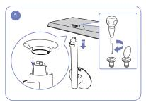
Insert the stand neck into the stand base in the direction shown in the figure. Tightly fasten the connecting screw at the bottom of the stand base.
