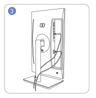
Connect the cables to their correct ports, and then arrange each of the two cables through either side of the COVER-STAND CABLE, as shown in the figure.
