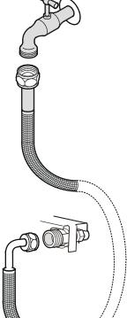
Connect the angled section of the stainless steel hose to the solenoid valve. The water connection to the appliance is via the solenoid valve on the rear of the appliance. The connection dimension is 3/4".
