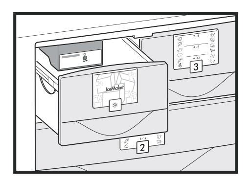
The ice maker is fitted in the freezer compartment of the combined refrigerator-freezer. It must be connected to the **mains water supply** to work. The descriptions below only relate to the ice maker and the water connection to a solenoid valve. All the instructions and details for the appliance as a whole are set out in the enclosed operating instructions for the combined refrigerator-freezer.
