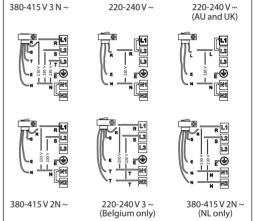
Connect the yellow/green earth wire to the terminal with the symbol  $\bigoplus$ . This wire must be longer than the other wires.
