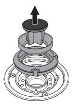
3. Pull the knobs and the knob bezels upwards to remove them.
