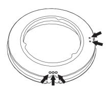
Refit the flame-spreader crowns making sure that they are correctly positioned in their housings with their respective burner caps.
