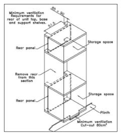
(Figure shows the ventilation and cut-out requirements for the installation of the appliance into a tall housing unit).
