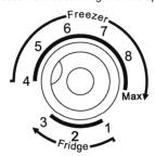
In positions 1 to 3, the appliance will operate as a refrigerator in approximate  $0^{\circ}$ C to  $10^{\circ}$ C. In positions 4 to max,the appliance will operate as a freezer in approximate -23°C to -10°C. If there is power light with your product, the POWER light on show the appliance is turned ON, light off show turned off The RUNNING light on show the compressor is operate.
