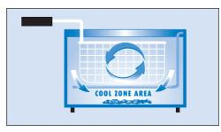
The submerged heating element system in the Deep Fryer allows oil to be heated more effectively, and respond quickly to oil temperature changes.
