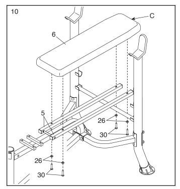
11. Attach the Seat (11) to the Frame (2) with four M6 x 40mm Screws (30) and four M6 Washers (26); start all the Screws, and then tighten them.
