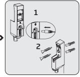
Install the end of the charging adaptor (19) to the seat on the back of the charging dock (15).
