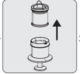
Remove the inlet foam inside the metal filter.
