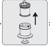
Remove the inlet foam inside the metal filter.
