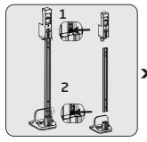
If you want to install the charging dock (15) to the wall, detach the charging unit from the tube (16) and support (17) using two separate buttons.
