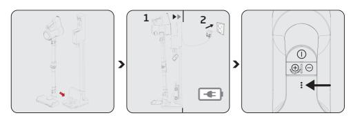
Secure the electric turbo brush (8) to the charging dock support.
