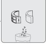
Remove the dust on the EPA E12 filter and outlet foam by tapping them to a hard surface such as a waste bin or by using a brush.
