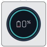
When you place the appliance to the charging dock (15), it starts to charge and the battery charge percentage shall be displayed on the screen (4). Percentage (%) and battery charge indicator are increased as the appliance is charged. The circle around the screen is illuminated in blue and as moving around.
