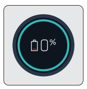
When you place appliance to the charging dock (15), it starts to charge and the battery charge percentage shall be displayed on the screen (4). Percentage (%) and battery charge indicator are increased as the appliance is charged. The circle around the screen is illuminated in blue and as moving around.
