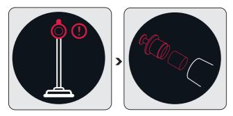
The filters shall be cleaned regularly to prevent loss of performance. When it is not cleaned regularly (in case of excessive dust), a filter cleaning animation is displayed on the screen for a very short period of time to indicate that the metal filter and inlet foam shall be cleaned. However, the appliance continues to operate.
