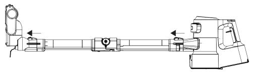
When you see the vacuum duct blockage warning on the screen (4), detach the brush (8) from the wand (6) to remove the blockages. Detach the wand (6) from the body of the appliance (10).
