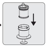
Remove the metal filter and inlet foam inside the dust reservoir (11) by rotating the metal filter counter-clockwise.
