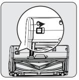
To remove the electric turbo brush (8), keep the roll brush release tab pressed so that the lock shall be opened in the direction of the arrow, rotate the roll cover towards yourself and pull it to the left.
