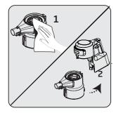
Install the metal filter inside the dust reservoir (11) by rotating it clockwise.
