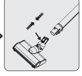
Press the electric turbo brush release button (7) on the electric turbo brush (8) and push it in the direction of arrow towards the wand.
