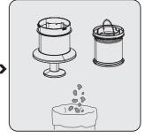
Remove the dust on the metal filter and inlet foam by tapping them to a hard surface such as a waste bin or by using a brush.
