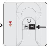
Press the "-" mode button (3) once to switch to a lower speed while operating at maximum speed or medium speed.
