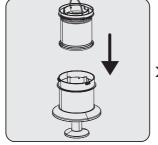
Install the dried inlet foam to the metal filter.
