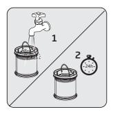
Wash the inlet foam under running cold water and let it dry.
