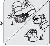
Push the trigger under the appliance to clean the dust reservoir (11).
