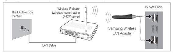
Samsung's Wireless LAN adapter is sold separately and is offered by select retailers, Ecommerce sites and Samsungparts.com. Samsung's Wireless LAN adapter supports the IEEE 802.11a/b/g and N communication protocols. Samsung recommends using IEEE 802.11n. When you play the video over a IEEE 802.11b/g connection, the video may not play smoothly.
