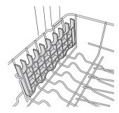
2 Locate assembly slot ① on cup rack and firmly pop rack off support bar on that side.
