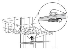
**7** After assembly, check whether the spray arms rotate freely.
