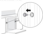
2 Drive a wood screw ( $\Phi$  4.5 x 12 mm) through the mounting bracket and into the cabinet frame.
