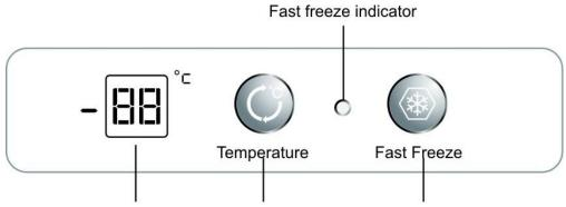
Digital display Temperature control key Fast freeze key
