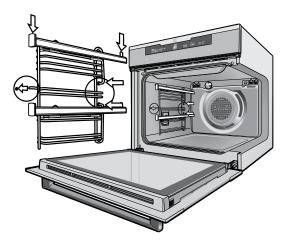
Note: If you have purchased an EVE623SA you will have additional side racks for the lower oven/grill. These are fitted in a similar manner, however the left hand side rack must be fitted to the lower two holes of the half cavity.
