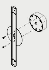
3. Raise the wall light and make the electrical connections inside the wall cover plate ensuring all wires are colour matched and the wall light is earthed correctly.
