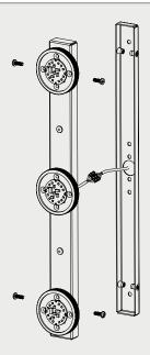
4 • Position on the back glass and fix into place by threading on the 3 x dome glass .
