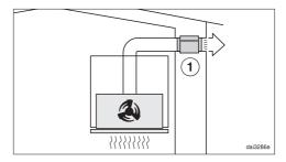
The silencer not only reduces noise from the motor outside the house, but also sounds from outside (e.g. traffic noise). For this reason, the silencer must be positioned as close as possible to the ducting exit ①.
