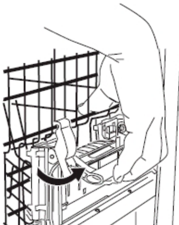
Fig. 6 Adjusting the rack for model DW60CDW2 / DW60CDX2
