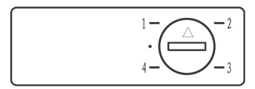
The temperature of the appliance can be adjusted by turning the thermostat dial.
