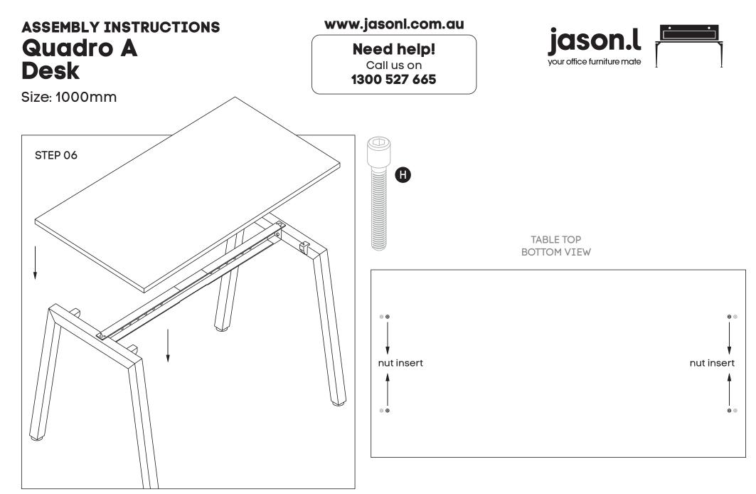
Place desktop ontop of frame. Nut inserts in top will align with plastic joiner brackets using M6x30MM **(H)** sockets attached top to frame.
