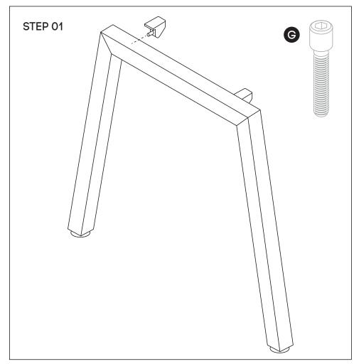
Using Allen Key provided, attach 2 plastic brackets per leg **(D)** (as per picture above) using M6x20MM **(G)** Socket head screw
