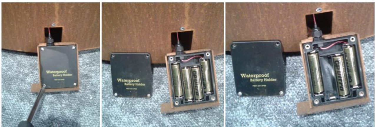
Photo 9: Replacing the batteries in the container
