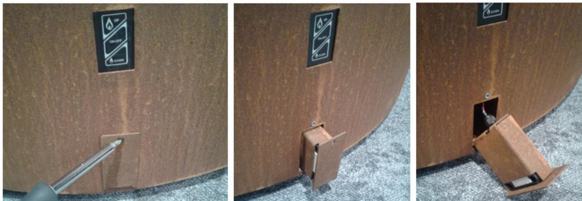
Photo 6: Removing of the battery container
