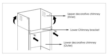
Drill 2 holes to accommodate the plate II. Screw and tighten the plate II onto the wall with two screws and wall.plugs provided Slide up the upper chimney and fix the upper chimney with plate II with 2 screws ST4x8mm
