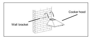
After hanging the hood on the bracket , remove the Alu Filters , mark 2 holes inside the hood for safety screws .After marking , remove
