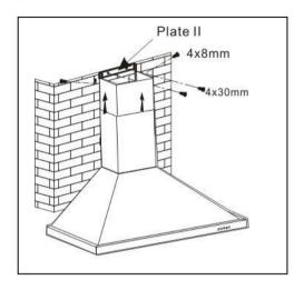
Fix the lower chimney with the hood with 2 screws ST4x8mm
