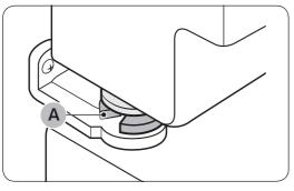
2. Insert a suitable-sized snap ring (A) between the door and the hinge as shown.
