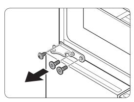
1. Remove the screw attached to the left and right middle hinges with a philips screwdriver (+). Remove the 2 hex head bolts attached to the left and right middle hinges with an allen spanner (Ø 4 mm).
