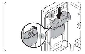
**3.** Reinsert the the upper door bin. check the water tank position if it is properly assembled.
