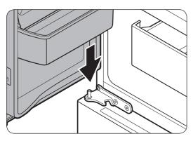
**1.** While holding the door open by more than 90 degrees, reinsert it into the middle hinge.
