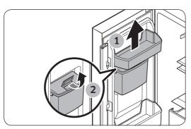
1. Remove the upper door bin first and open the water tank cover.
