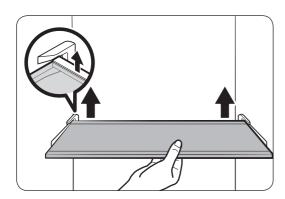
• Slightly lift up the rear side of the shelf to pull out.
