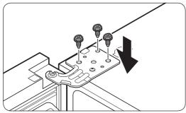
**4.** Insert and tighten the 3 hex head bolts into the left and right upper hinges with a socket wrench (8 mm).
