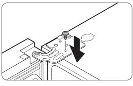
**3.** Insert and tighten the ground screw into the left and right upper hinges with a Phillips screwdriver (+).
