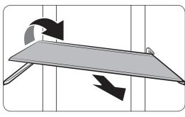
• Twist the shelf diagonally to remove.
