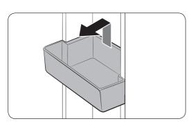
To remove the top door bin, hold the front sides of the bin, and then gently lift up to remove.
