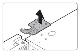
2. Disconnect electric wire on the top of the refrigerator.
