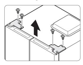
1. With the door closed, use a Phillips screwdriver to remove the screws (x4) from the cover hinge. Pull up and remove the top cover with the connectors.
