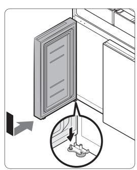
**1.** Insert the freezer door into the bottom hinge while pushing the freezer door in the arrow direction.
