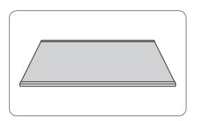
To secure more room in the **freezer** remove the **middle drawer** of the **freezer**, and then insert the **freezer shelf** between the middle and bottom drawers.
