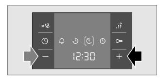
After a few seconds, the oven adopts the settings and switches to standby position. The display shows the time at which the dish will be ready and the symbol & is in brackets. The A and B symbols go out. When the oven starts, the cooking time counts down in the display and the Symbol is shown in brackets. The symbol & goes out.
