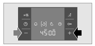
The main oven will start up after a few seconds. In the display, the timer period counts down and the symbol [3] lights up. The other time symbols go out.
