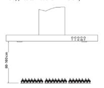
Install the hood centrally over the cooktop. Mount the hood bottom between 800 to 1000mm above the cooktop. Mark the position for drilling of the fixing bolts.
