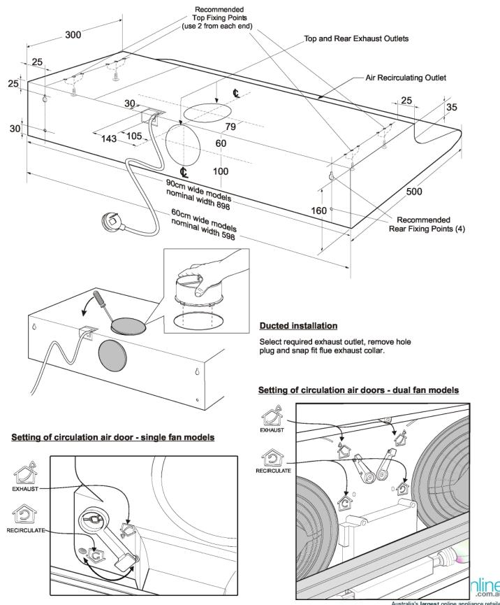
Australia's largest online appliance retailer IMPORTANT: SET CIRCULATING MODES BEFORE INSTALLING THE HOLE PLUGS.
