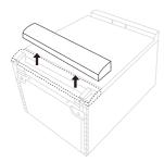
3 Remove the double-sided tape on the back of the felt and attach it to the front side of the appliance's bottom.
