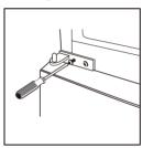
7. Unscrew right middle stopper with metal block from bottom of upper door. And then install left middle stopper and metal block in left side of bottom of upper door.
