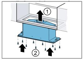
2. Tighten the fastening screws.
