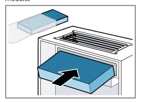
3. Fit the panel such that it is held firmly in place by the magnets.
