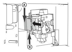
**N.B.:** If you encounter difficulty inserting the brewing unit, before inserting it adapt it to the right size by pressing it forcefully from both the bottom and top simultaneously as shown in the figure.
