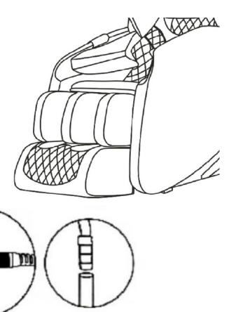
Connect the cable line if not connected.
