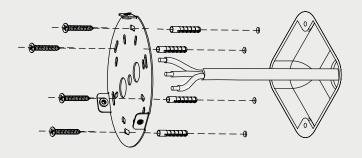
2. Bring the body of the light closer to the mounting plate and make the electrical connections within wall rose, ensuring all wires are colour matched and the pendant is earthed correctly.
