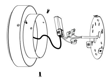
$\ensuremath{\mathsf{A}}.$  Make power connection to the LED driver. See wiring diagram.
