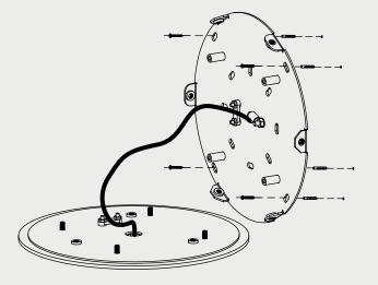
5. Attach the gear tray back to the mounting plate by using the flat head screws (A), you removred on step 2.
