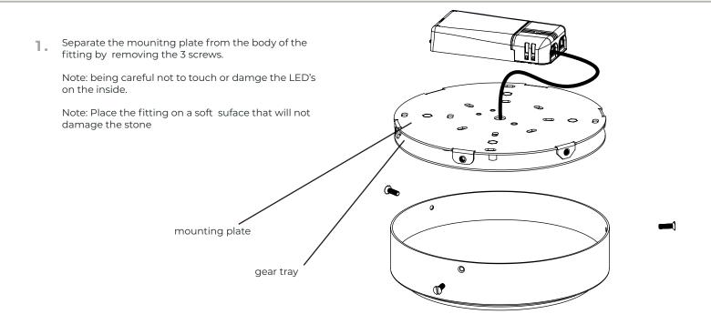
2. Separate the gear tray from the mounting plate.
