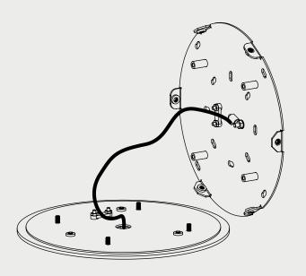
**3**. Fit the driver into the cavity of wall or ceiling.
