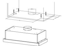
respecting the distance indicated. Push the hood up against the wall unit and insert the 4 screws operating from inside the wall unit
