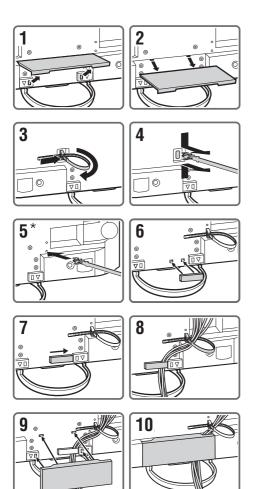
\* When installing on the wall, attach the cable holder under the terminals.
