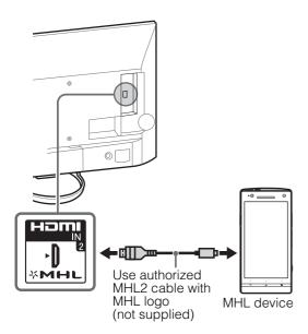
The MHL (Mobile High-Definition Link) enables the TV to communicate with a connected MHL-compatible device. The TV can charge the connected MHL-compatible device while playing photo/music/video from it. You can use the TV remote control to control the connected MHL-compatible device.
