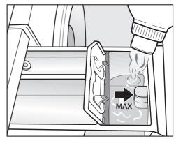
■ Add fabric softener or liquid starch to the ⊗ compartment. **Do not exceed** the maximum level mark.
