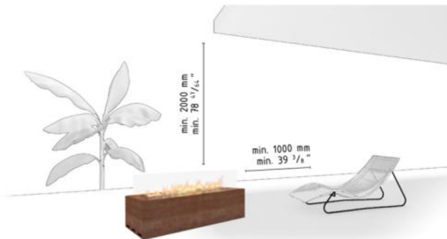
Figure 1: Minimum distance to flammable materials
