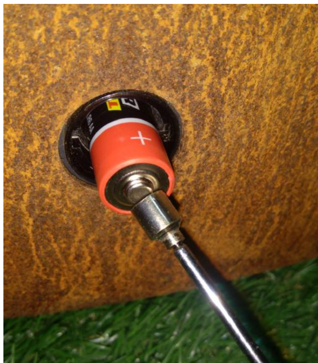
Photo 7: Removing the first battery using the magnetic gripper
