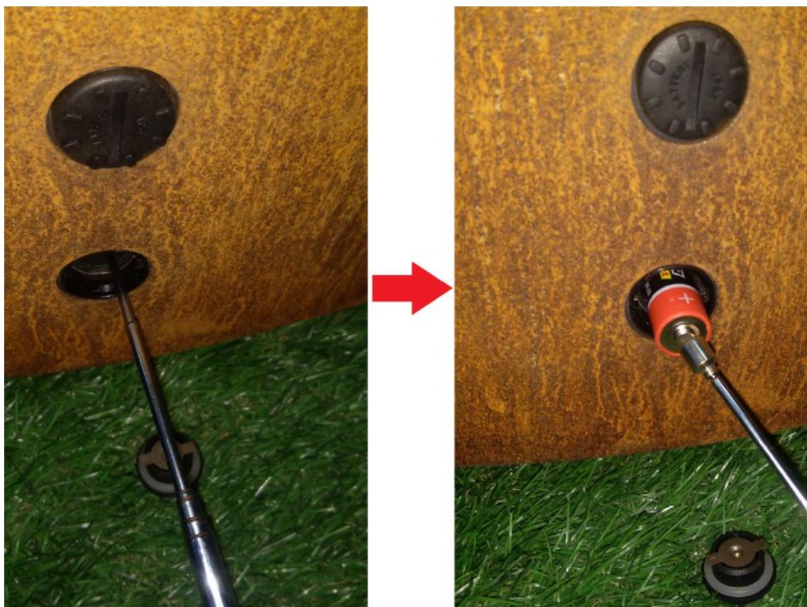
Photo 8: Removing the second battery from the container
